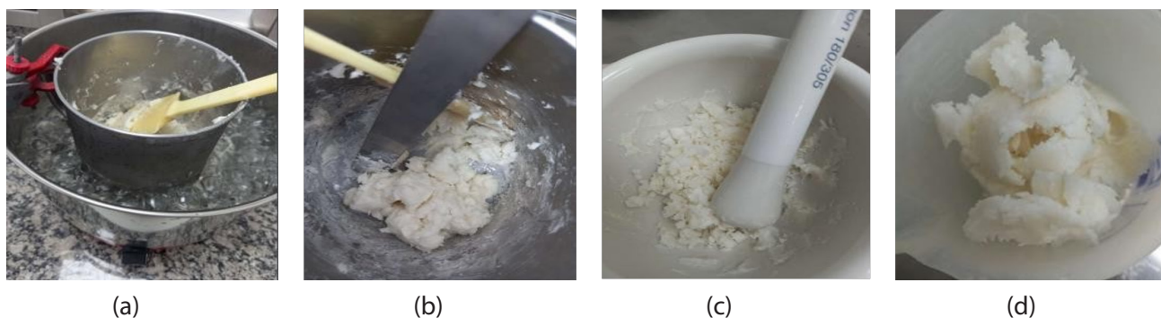
Figure 1 - A mixture of sodium isethionate and cocoamidopropyl betaine. (a) The image shows the heating performed in a water bath. (b) Paste formation of sodium isethionate and cocoamidopropyl betaine. (c) Paste of sodium isethionate and cocoamidopropyl betaine being milled. (d) Paste after shredding.
